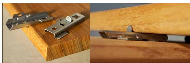
Fasten the Spezialfix with the integrated assembly stop on the back of the decking board using two 4.2 x 17 mm stainless steel screws. Fasten the next special fix on the opposite side offset. Then turn the decking board around and fasten it with a special clip on the substructure using a 4.2 x 35 mm stainless steel screw. Repeat this process with the next floorboards. Fasten the start and end board visibly from above using stainless steel screws.
