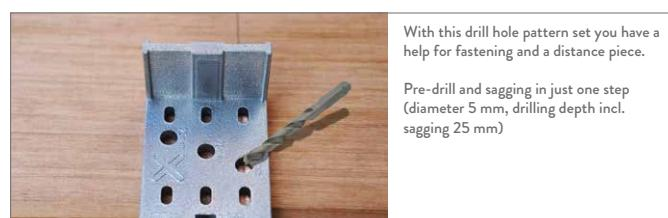
With this drill hole pattern set you have a help for fastening and a distance piece.
